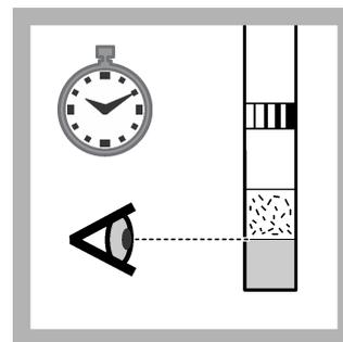
4. Then leave the cuvette to stand. Wait for the phase separation to finish (**approximately 2 minutes**).
