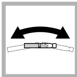
3. Hold the cuvette between thumb and index finger. **Mix intensively** (2–3 times per second) for **2 minutes** – **do not shake**.
