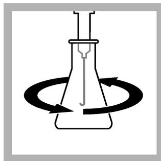
11. Put the end of the delivery tube fully into the solution. Swirl the flask. Turn the knob on the Digital Titrator to add titrant to the solution. Continue to swirl the flask. Add titrant until the color changes from red to pure blue. Record the number of digits on the counter.
