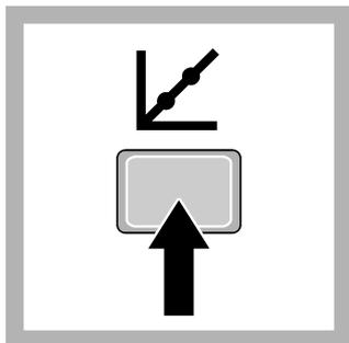
6. Push **Calibrate**. The standard solution value is shown.
