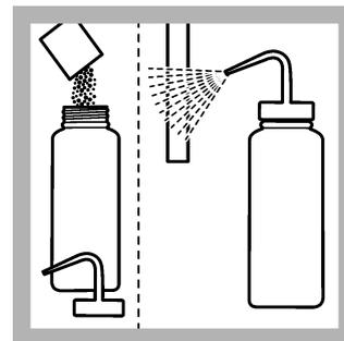
8. Rinse the probe with ISA rinse solution. Do not rinse with deionized water. Dry the probe with a lint-free cloth.
