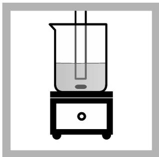
5. Put the probe in the solution. Do not let the probe touch the stir bar, bottom or sides of the container. Make sure that the reference junctions are fully in the solution. Remove the air bubbles from under the probe tip.
