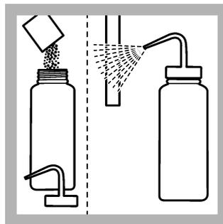
7. Rinse the probe with ISA rinse solution. Do not rinse with deionized water. Dry the probe with a lint-free cloth.
