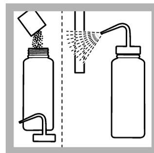
4. Rinse the probe with ISA rinse solution. Do not rinse with deionized water. Dry the probe with a lint-free cloth.
