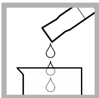
1. Add 25 mL of 10-mg/L Sodium Standard Solution to a beaker.
