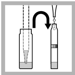
6. **Slowly** pipet into the Cuvette Test: **0.5 mL** of digested sample.
